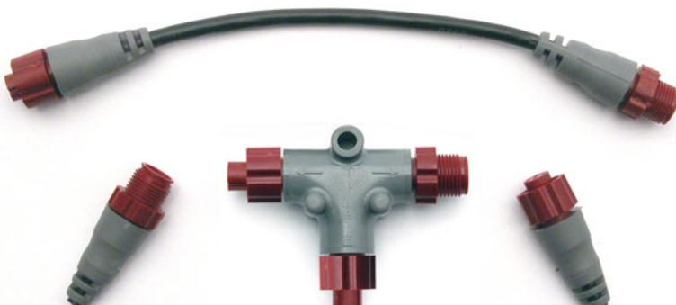
**LowranceNET Node Kit for a NMEA 2000 network. Includes a 2 foot (61 cm) extension cable, T connector, 120-ohm male terminator and 120-ohm female terminator.**
