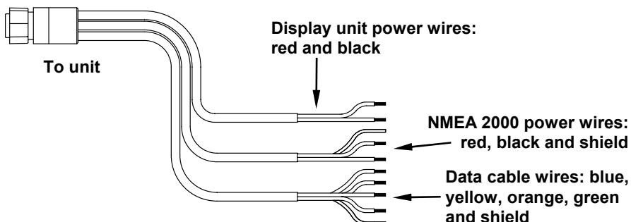
**The Power/Data cable for the display unit used with the GPS module.**
